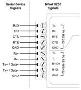
Note: NPort 5232/5232I has 2 RS-422/485 ports. The pin assignments are the same as NPort 5230's port 2. Refer to the "NPort 5200 Series User's Manual" for more details
