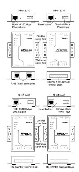
Reset Button—Press the *Reset button* continuously for 5 sec to load factory defaults: Use a pointed object, such as a straightened paper clip or toothpick, to press the reset button. This will cause the Ready LED to blink on and off. The factory defaults will be loaded once the Ready LED stops blinking (after about 5 seconds). At this point, you should release the reset button.
